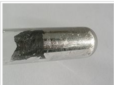
Indium wetting the glass surface of a test tube
